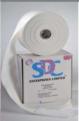
It is produced with a narrow weave construction and contains the following components: secondary cellulose acetate, cotton, polyamide, polyester, acrylic and wool.
