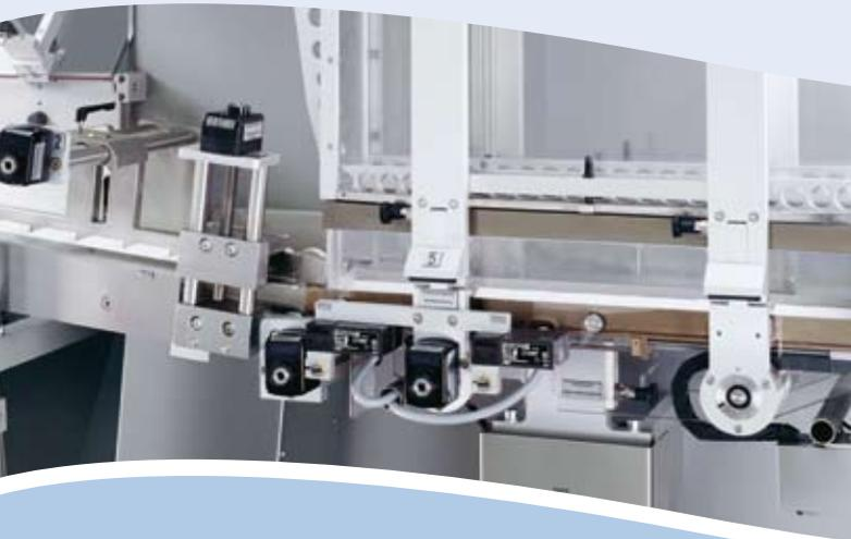
Film unwind with cross pushing function and sealing station
