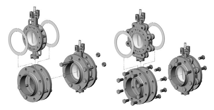
**DANGER:** When installing the butterfly valve with flanged body used in an end-of-line function, the free connection side must be additionally secured by a blind flange or (only for short-term use) the valve must be locked tightly in the "CLOSED" position. Only manual operations that are self-locking like gear operators for valves are allowed. Hand levers with notch plates do not fulfil this function!
