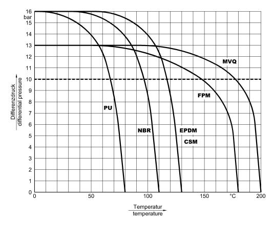
From DN 200 the use of seats with higher shore hardness is necessary at a differential pressure of more than 13 bar. Lug type valves: Max. differential pressure 6 bar for valves used in an end-of-line function. KG2 / KG4 and valves from DN 600: Max. differential pressure 10 bar.
