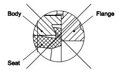
Remove the flange-spreaders and tighten the flange screws slightly and evenly <u>crosswise</u> with the disc fully opened.
